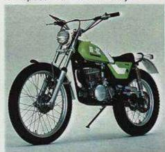
Rear suspension units are adjustable and double-acting to provide excellent damping and control even over the most difficult terrain.
