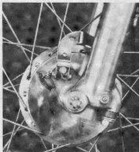
The front brake arm is cleverly designed so that it is not vulnerable. This setup also allows the front brake cable to be routed behind the left fork leg.
