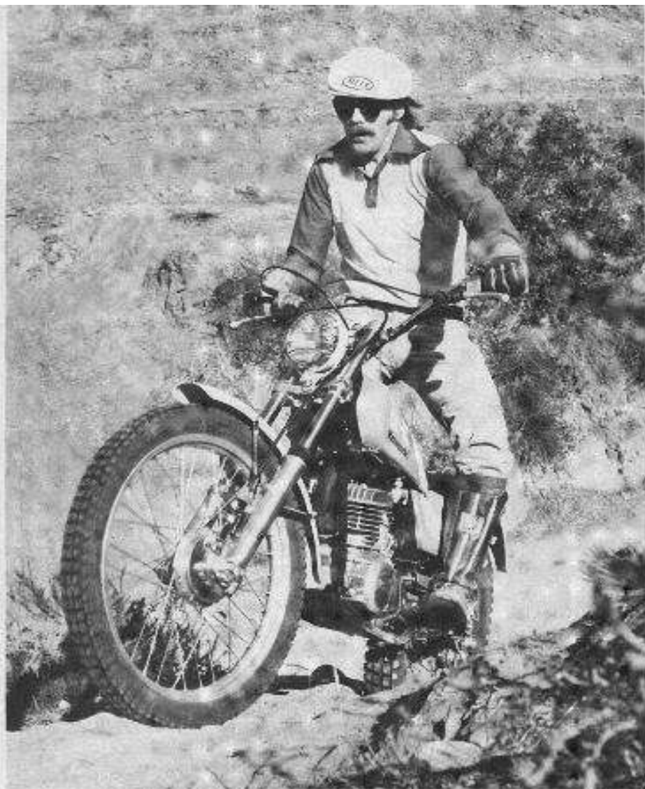
The control cables are much too long, causing them to snag frequently on bushes or tree branches.
