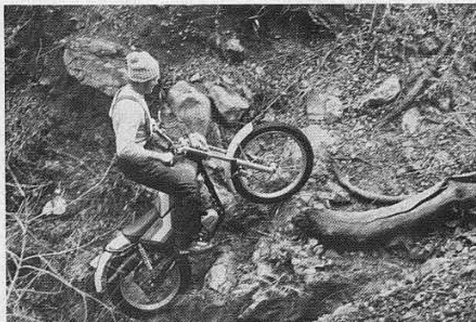
Trying for a progressive spring rate by using two different springs doesn't make it. In any case the springing is too soft both front and rear.
