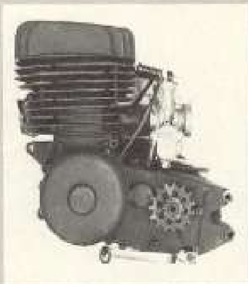
Three views of the latest big bore Kawasaki motocross engine. Just about everything but the transmission case is made from aluminum, except the cylinder barrel, which is aluminum. Dry weight of the engine is 62 lbs.
